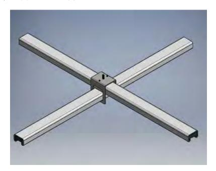
Crossovers provide the mechanical connection for building runs, rows, and grids. One universal crossover serves as an X, T, or an L intercept. The ONE over ONE crossover is used when one single-deck length of busSTRUT intersects another single-deck length of busSTRUT.
